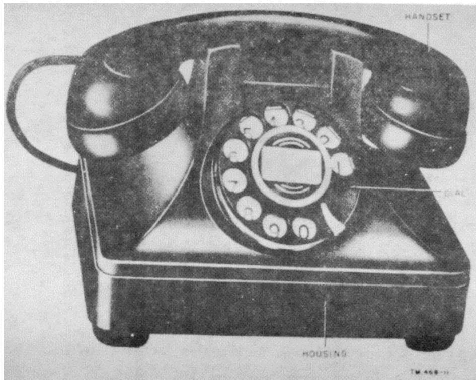
Figure 10. Telephone TP-6 (North Elec Mfg No. H-600SL), arranged for dial operation
